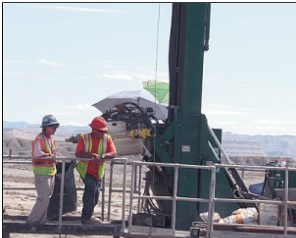
Drill rig operators collect soil samples.
